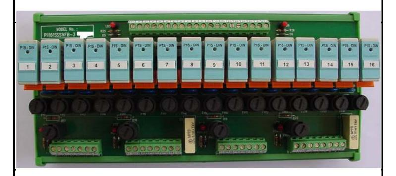
These Relay modules provide a compact, reliable & cost effective means of providing an isolation and safety barrier between the field equipment and the PLC
